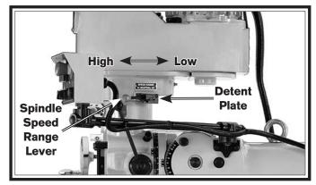
Figure 34. Spindle speed range selector.
